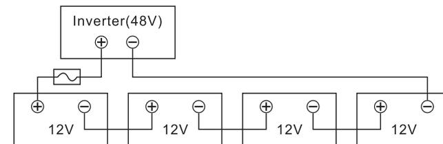
2. Insert the battery wires flatly into battery connectors of inverter and make sure the bolts are tightened with torque of 2 Nm in clockwise direction. Make sure polarity at both the battery and the inverter/charge is correctly connected and conductors are tightly screwed into the battery terminals. Recommended tool: # 2 Pozzi Screwdriver
