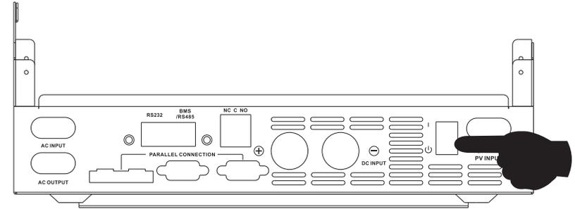
Once the unit has been properly installed and the batteries are connected well, simply press On/Off switch (located on the button of the case) to turn on the unit.
