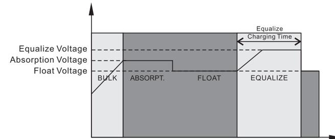
However, in Equalize stage, when battery equalized time is expired and battery voltage doesn't rise to battery equalization voltage point, the charge controller will extend the battery equalized time until battery voltage achieves battery equalization voltage. If battery voltage is still lower than battery equalization voltage when battery equalized timeout setting is over, the charge controller will stop equalization and return to float stage.
