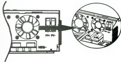
4. Check correct polarity of wire from PV modules and PV input connectors. Then, connect positive pole (+) of connection wire to positive pole (+) of PV input connector. Connect negative pole (-) of connection wire to negative pole (-) of PV input connector. Screw two wires tightly in clockwise direction. Recommended tool: 4mm blade screwdriver.
