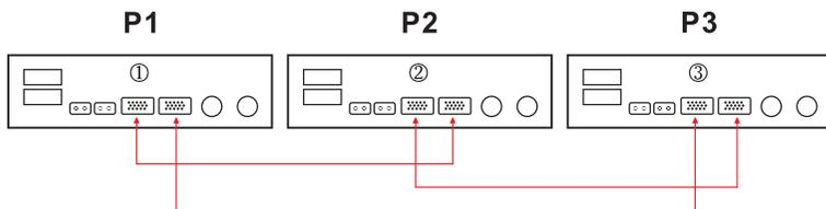
**WARNING:**Do not connect the current sharing cable between the inverters which are in different phases. Otherwise, it may damage the inverters.
