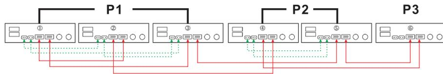
Three inverters in one phase and only one inverter for the remaining two phases:
