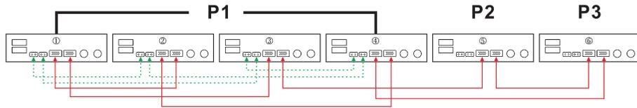
Three inverters in one phase, two inverters in second phase and one inverter for the third phase:
