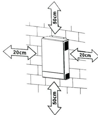
**! SUITABLE FOR MOUNTING ON CONCRETE OR OTHER NON-COMBUSTIBLE SURFACE ONLY.**
