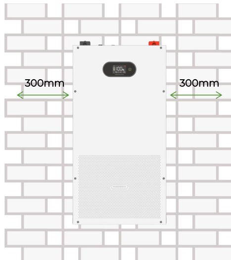
Figure 3-3 Mounting Space Requirements
