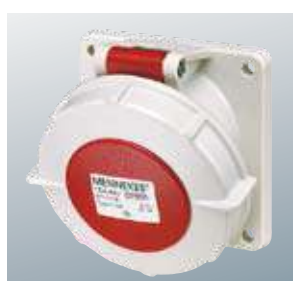
⚠ IP 67 CEE panel mounted receptacles, screwless, with TwinCONTACT, standard flange dimensions 85 x 85 mm, 20° inclination Dimensions: page 71
