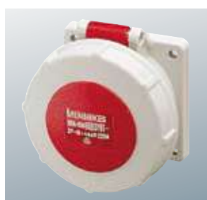
⚠ IP 67 CEE panel mounted receptacles, screwless, with TwinCONTACT, flange: 16A: 75 x 75 mm, 32A: 85 x 75 mm, straight Dimensions: page 70/71
