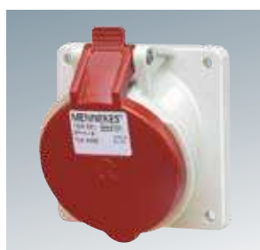
⚠ IP 44 CEE panel mounted receptacles, screwless, with TwinCONTACT, standard flange dimensions 85 x 85 mm, 20° inclination Dimensions: page 70/71
