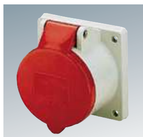
⚠ IP 44 CEE panel mounted receptacles, screwless, with TwinCONTACT, flange: 75 x 75 mm, straight Dimensions: page 70/71
