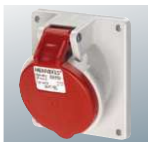
⚠ IP 44 CEE panel mounted receptacles, screwless, with TwinCONTACT, flange: 16A, 3p: 73.5 x 64 mm, 16A, 4+5 p, 32A: 100 x 92 mm, 20° inclination Dimensions: page 70/71
