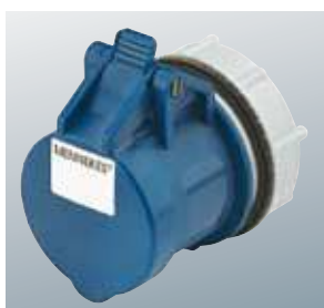
⚠ IP 44 CEE panel mounted receptacles RAPIDO, screwless, with TwinCONTACT Dim.: page 70/71 with central locking system, round flange for central fixing, dia. 61 mm
